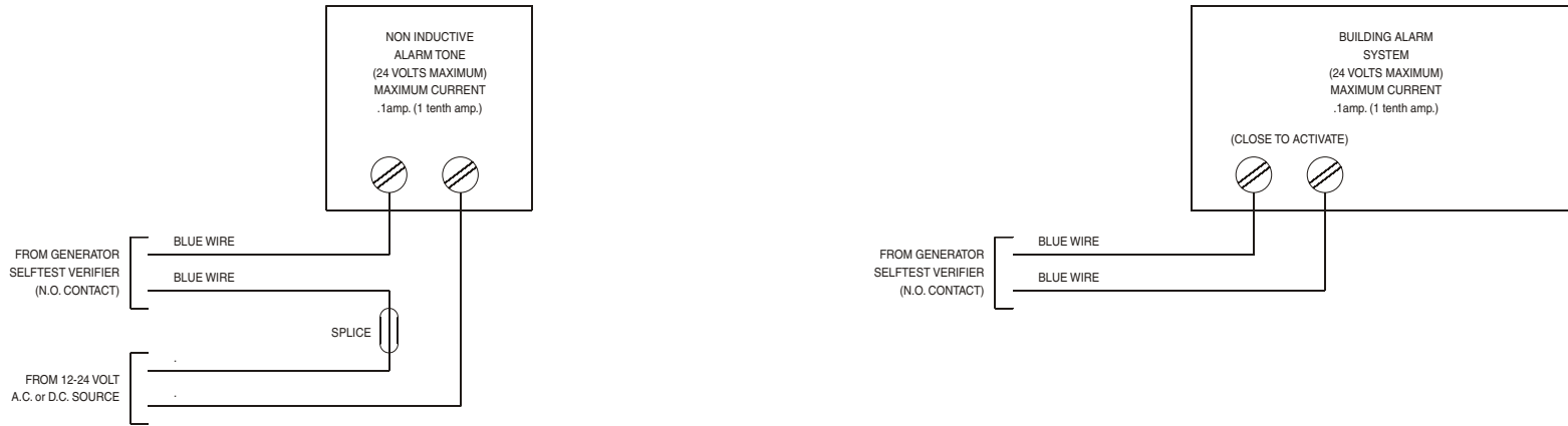
FIGURE 6 OF 6 WIRING DIAGRAMS FOR REMOTE ALARMS UNDER .1amp. (1 tenth amp.)
